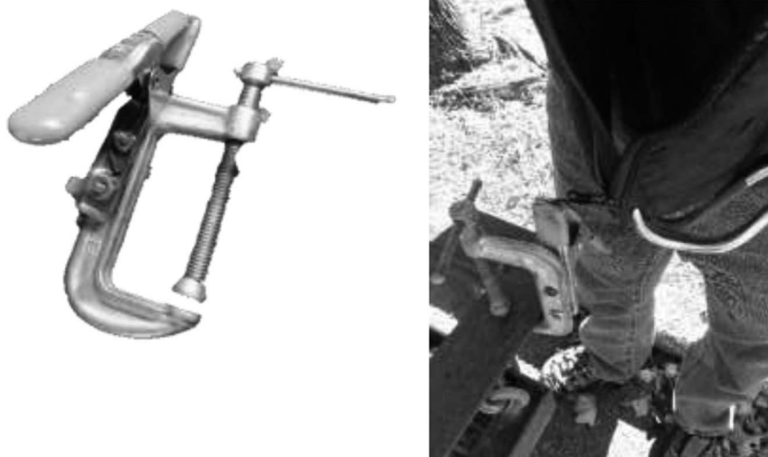
Figure 17. A, A homemade “extra hand/zipper holder” is attached with the carpenter’s clamp onto a countertop or other sturdy object; then the strong clamp can be used to pinch onto whatever needs to be pinched. B, A zipper pull is gripped while the terminal device pulls the garment down (photograph courtesy John Krenzel).
